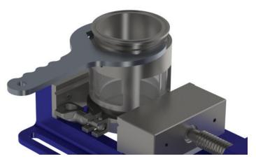
Using supplied Dixon wrench, rotate the sight glass top cap clockwise for assembly or counterclockwise for disassembly.
